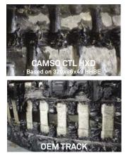
After 196 hours of testing, the competitor's tracks failed. Camso's tread was in good condition on the entire track.
