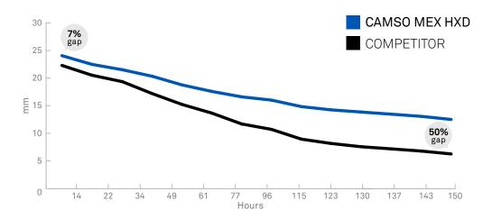
Camso tracks are designed with much thicker tread than most OEM tracks. Maintaining more rubber around the carcass offers more protection on carcass puncture and edge cutting. This all translates in longer service life and less downtime. The end result of this test is:
